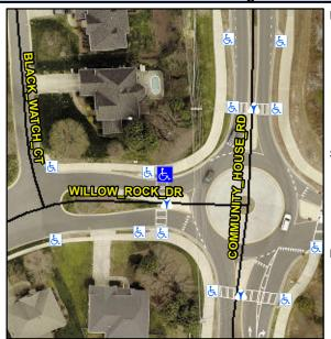
WILLOW ROCK DR Street 1 Name Stop Condition-Street 1 YieldSign Street 2 Name N/A Stop Condition-Street 2 N/A Possible Solutions: Remove & Replace Curb Ramp With **Two New Directional Ramps or** Equivalent. Surveyor Notes: N/A PROW/ADA: R304.5.3
