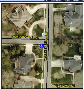
WHITNEY HILL RD Street 1 Name Stop Condition-Street 2 Street 2 Name **GORDONVALE PL** Stop Condition-Street 1 StopSign Possible Solutions: Co **Remove & Replace Curb Ramp With** N/ **Two New Directional Ramps or** Ye Equivalent. Surveyor Notes: N/A PROW/ADA: R304.2.2, R304.5.3
