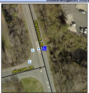
STATESVILLE RD Street 1 Name Stop Condition-Street 1 None N/A Street 2 Name Stop Condition-Street 2 N/A Possible Solutions: Remove & Replace Detectable Warning System. Relocate Obstruction. Surveyor Notes: NO CURB, NO SW, DWS OS **MEASRUED TO ASP** PROW/ADA: R305.1.4, R305.2, R302.3, R402.2
