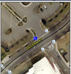
**GALLERIA BV** Street 1 Name Stop Condition-Street 2 None Street 2 Name **ENTRANCE** Stop Condition-Street 1 None Possible Solutions: Remove & Replace Curb Ramp With **Two New Directional Ramps or** Equivalent. Surveyor Notes: N/A PROW/ADA: R304.5.1
