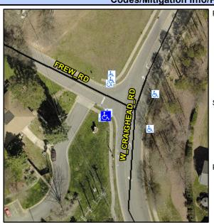
Street 1 Name Stop Condition-Street 1 Street 2 Name Stop Condition-Street 2 W CRAIGHEAD RD Possible Solutions: Remove & Replace Curb Ramp With Two New Directional Ramps or Equivalent. Surveyor Notes: N/A PROW/ADA: Not Found, R304.5.1, R304.5.3, R304.3.2
