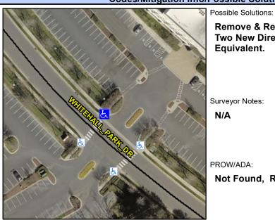
WHITEHALL PARK DR Street 1 Name Stop Condition-Street 1 None Street 2 Name N/A Stop Condition-Street 2 StopSign **Remove & Replace Curb Ramp With** Two New Directional Ramps or Equivalent.
