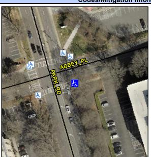
**ABBEY PL** Street 1 Name Stop Condition-Street 2 Signal **PARK RD** Street 2 Name Stop Condition-Street 1 Signal Possible Solutions: Compliance Description N/A Remove & Replace Curb Ramp With Two New Directional Ramps or Yes Equivalent. Restripe Crosswalk. N/A N/A N/A N/A Surveyor Notes: N/A N/A N/A PROW/ADA: Not Found, R304.2.2
