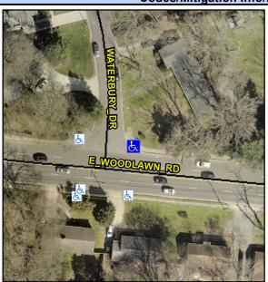
StopSign Street 1 Name Stop Condition-Street 1 WATERBURY DR Street 2 Name Stop Condition-Street 2 E WOODLAWN RD Possible Solutions: Remove & Replace Curb Ramp With Two New Directional Ramps or Equivalent. Surveyor Notes: ASP LIP 2.0 PROW/ADA: Not Found, R304.5.1, R304.3.2
