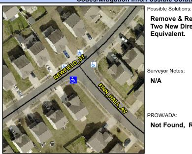
Street 1 Name Stop Condition-Street 2 Street 2 Name Stop Condition-Street 1 **FINN HALL AV** StopSign **NEWFIELD ST** None Remove & Replace Curb Ramp With Two New Directional Ramps or Equivalent.
