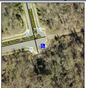
FRIENDSHIP VILLAGE PL Street 1 Name Stop Condition-Street 2 None **MISSIONARY AV** Street 2 Name Stop Condition-Street 1 None Possible Solutions: Compliance Description N/A Remove & Replace Curb Ramp With Two New Directional Ramps or No Equivalent. Surveyor Notes: N/A PROW/ADA: Not Found, R304.5.1, R304.2.2
