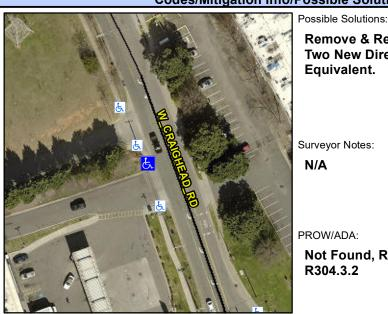
Street 1 Name Stop Condition-Street 1 Street 2 Name Stop Condition-Street 2 Two New Directional Ramps or Equivalent.
