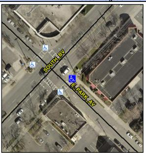
Street 1 Name Stop Condition-Street 1 Street 2 Name Stop Condition-Street 2 Possible Solutions: Remove & Replace Curb Ramp With Two New Directional Ramps or Equivalent.
