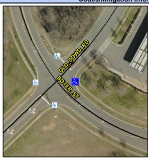
**OLD DOWD RD** Street 1 Name Stop Condition-Street 1 StopSign **BOYER ST** Street 2 Name Stop Condition-Street 2 None Remove & Replace Curb Ramp With Two New Directional Ramps or Equivalent.
