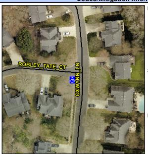
**ROBLEY TALE CT** Street 1 Name Stop Condition-Street 2 None **OXWYNN LN** Street 2 Name Stop Condition-Street 1 None Possible Solutions: Remove & Replace Curb Ramp With Two New Directional Ramps or Equivalent. Surveyor Notes: N/A PROW/ADA: Not Found, R304.5.1, R304.2.2
