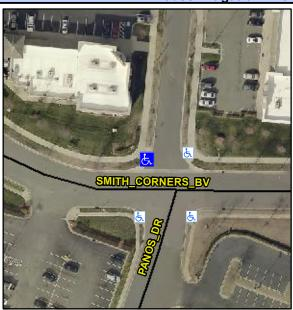
**SMITH CORNERS BV** Street 1 Name Stop Condition-Street 1 **PANOS DR** Street 2 Name Stop Condition-Street 2 StopSign Possible Solutions: Remove & Replace Curb Ramp With Two New Directional Ramps or Equivalent. Surveyor Notes: N/A PROW/ADA: Not Found, R304.5.3
