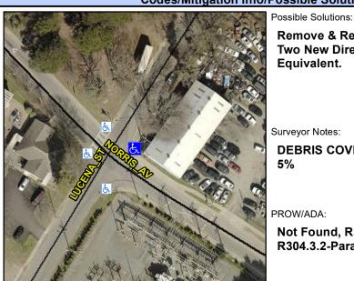
Street 1 Name Stop Condition-Street 1 Street 2 Name Stop Condition-Street 2 **LUCENA ST** StopSign **NORRIS AV** None Remove & Replace Curb Ramp With Two New Directional Ramps or Equivalent.
