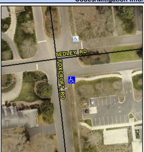
**SEDLEY RD** Street 1 Name Stop Condition-Street 2 StopSign Street 2 Name **FOXCROFT RD** Stop Condition-Street 1 StopSign Possible Solutions: Remove & Replace Curb Ramp With **Two New Directional Ramps or** Equivalent. Surveyor Notes: N/A PROW/ADA: Not Found, R304.2.2, R304.5.3
