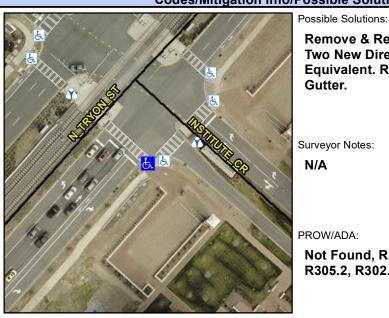
N TRYON ST Street 1 Name Stop Condition-Street 1 Signal Street 2 Name N/A Stop Condition-Street 2 N/A Remove & Replace Curb Ramp With Two New Directional Ramps or Equivalent. Remove & Replace Gutter.
