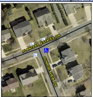
Street 1 Name Stop Condition-Street 2 Street 2 Name Stop Condition-Street 1 **PLANTERS ESTATES DR** None **SUNRISE VIEW DR** StopSign Possible Solutions: Remove & Replace Curb Ramp With **Two New Directional Ramps or** Equivalent. Surveyor Notes: N/A PROW/ADA: R304.5.1, R304.2.2, R304.5.3
