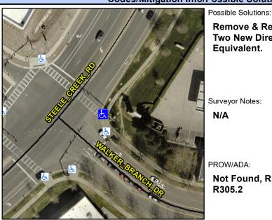
STEELE CREEK RD Street 1 Name Stop Condition-Street 1 Signal Street 2 Name N/A Stop Condition-Street 2 N/A **Remove & Replace Curb Ramp With Two New Directional Ramps or** Equivalent.
