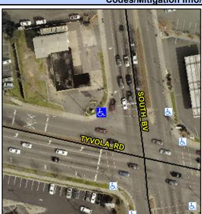
**TYVOLA RD** Street 1 Name Stop Condition-Street 2 Signal **SOUTH BV** Street 2 Name Stop Condition-Street 1 Signal Possible Solutions: Remove & Replace Curb Ramp With Two New Directional Ramps or Equivalent. Surveyor Notes: N/A PROW/ADA: R304.2.2
