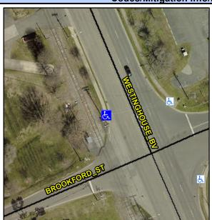
**WESTINGHOUSE BV** Street 1 Name Stop Condition-Street 1 None Street 2 Name N/A Stop Condition-Street 2 N/A Possible Solutions: Remove & Replace Entire Ramp. Surveyor Notes: N/A PROW/ADA: R304.5.3, R304.3.2
