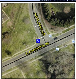
Street 1 Name Stop Condition-Street 2 Street 2 Name Stop Condition-Street 1 E ARROWOOD RD None KINGS RIDGE DR StopSign Possible Solutions: Remove & Replace Curb Ramp With **Two New Directional Ramps or** Equivalent. Surveyor Notes: N/A PROW/ADA: R304.5.1, R304.2.2, R304.5.3
