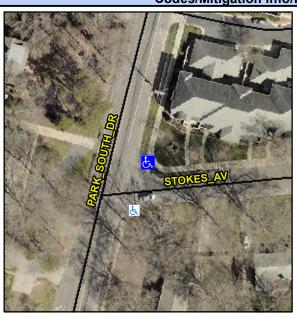
Street 1 Name Stop Condition-Street 2 Street 2 Name Stop Condition-Street 1 PARK SOUTH DR None STOKES AV StopSign Possible Solutions: Remove & Replace Curb Ramp With **Two New Directional Ramps or** Equivalent. Surveyor Notes: N/A PROW/ADA: Not Found, R304.5.1, R304.2.2, R304.5.3
