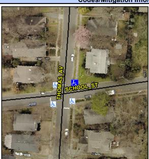
**THOMAS AV** Street 1 Name Stop Condition-Street 2 StopSign **SCHOOL ST** Street 2 Name Stop Condition-Street 1 StopSign Possible Solutions: Remove & Replace Curb Ramp With **Two New Directional Ramps or** Equivalent. Surveyor Notes: N/A PROW/ADA: Not Found, R304.5.1
