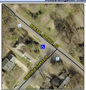
Street 1 Name None Stop Condition-Street 1 CARRIAGE OAKS DR Street 2 Name N/A Stop Condition-Street 2 N/A Possible Solutions: Remove & Replace Entire Ramp. Surveyor Notes: LT RP < 5% PROW/ADA: R304.5.1, R304.2.2, R304.5.3, R304.3.2
