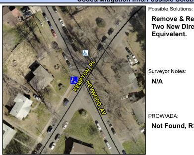
**HEYWOOD AV** Street 1 Name Stop Condition-Street 1 StopSign Street 2 Name N/A Stop Condition-Street 2 N/A Remove & Replace Curb Ramp With **Two New Directional Ramps or** Equivalent.
