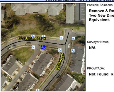
Street 1 Name **BRISTLE TOE LN** Stop Condition-Street 2 None Street 2 Name N/A Stop Condition-Street 1 None **Remove & Replace Curb Ramp With Two New Directional Ramps or** Equivalent.
