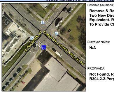
E MARTIN LUTHER KING JR BV Street 1 Name Signal Stop Condition-Street 2 Street 2 Name S DAVIDSON ST Stop Condition-Street 1 Signal Remove & Replace Curb Ramp With Two New Directional Ramps or Equivalent. Restripe Crosswalk(s) To Provide Clear space.
