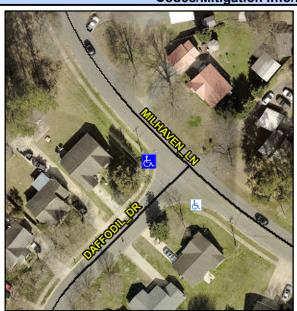
**DAFFODIL DR** Street 1 Name Stop Condition-Street 1 StopSign Street 2 Name N/A Stop Condition-Street 2 N/A Remove & Replace Curb Ramp With Two New Directional Ramps or Equivalent.
