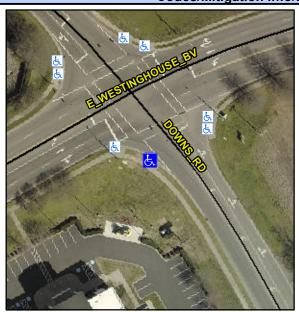
**DOWNS RD** Street 1 Name Stop Condition-Street 2 Signal Street 2 Name N/A Stop Condition-Street 1 N/A Possible Solutions: Remove & Replace Entire Ramp. Restripe Crosswalk. Surveyor Notes: N/A PROW/ADA: Not Found, R304.2.2, R304.5.3
