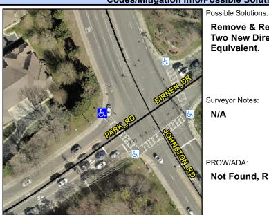
**PARK RD** Street 1 Name Stop Condition-Street 2 Signal Street 2 Name **JOHNSTON RD** Stop Condition-Street 1 Signal Remove & Replace Curb Ramp With Two New Directional Ramps or Equivalent.
