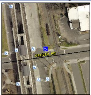
**ENTRANCE** Street 1 Name Stop Condition-Street 2 None Street 2 Name **ENTRANCE** Stop Condition-Street 1 None Possible Solutions: Remove & Replace Curb Ramp With Two New Directional Ramps or Equivalent. Surveyor Notes: N/A PROW/ADA: Not Found, R304.5.3
