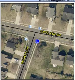
DAVID COX RD Street 1 Name Stop Condition-Street 1 **SACKETT WY** Street 2 Name Stop Condition-Street 2 StopSign Possible Solutions: Remove & Replace Curb Ramp With Two New Directional Ramps or Equivalent. Surveyor Notes: N/A PROW/ADA: R304.5.1, R304.5.3
