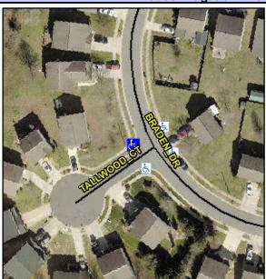
Street 1 Name Stop Condition-Street 2 Street 2 Name Stop Condition-Street 1 **TALLWOOD CT** StopSign **BRADEN DR** None Possible Solutions: Remove & Replace Curb Ramp With **Two New Directional Ramps or** Equivalent. Surveyor Notes: N/A PROW/ADA: Not Found, R304.5.3
