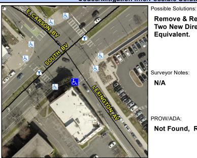
**LEXINGTON AV** Street 1 Name Stop Condition-Street 1 Signal Street 2 Name N/A Stop Condition-Street 2 N/A Remove & Replace Curb Ramp With **Two New Directional Ramps or** Equivalent.
