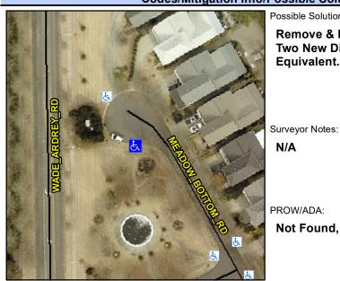
Street 1 Name Stop Condition-Street 2 Street 2 Name Stop Condition-Street 1 **MEADOW BOTTOM RD** None **MEADOW BOTTOM RD** None Possible Solutions: Remove & Replace Curb Ramp With **Two New Directional Ramps or** Equivalent.
