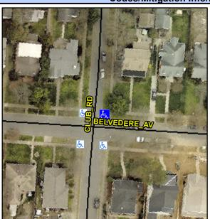
**CLUB RD** Street 1 Name Stop Condition-Street 2 StopSign **BELVEDERE AV** Street 2 Name Stop Condition-Street 1 None Possible Solutions: Compliance Description Remove & Replace Curb Ramp With Two New Directional Ramps or Equivalent. Surveyor Notes: N/A PROW/ADA: R304.5.1
