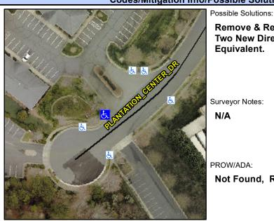
PLANTATION CENTER DR Street 1 Name Stop Condition-Street 2 None **ENTRANCE** Street 2 Name Stop Condition-Street 1 StopSign Remove & Replace Curb Ramp With Two New Directional Ramps or Equivalent.
