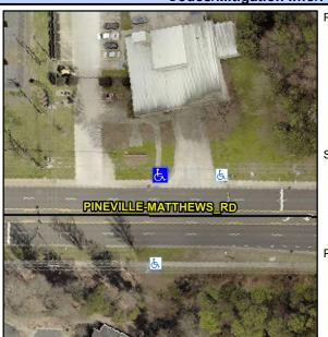
PINEVILLE-MATTHEWS RD Street 1 Name Stop Condition-Street 2 None Street 2 Name **ENTRANCE** Stop Condition-Street 1 None Possible Solutions: Remove & Replace Curb Ramp With Two New Directional Ramps or Equivalent. Surveyor Notes: N/A PROW/ADA: Not Found, R304.2.2
