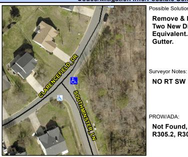
**SOUTHMINSTER LN** Street 1 Name Stop Condition-Street 1 StopSign Street 2 Name N/A Stop Condition-Street 2 N/A Possible Solutions: Remove & Replace Curb Ramp With Two New Directional Ramps or Equivalent. Remove & Replace Gutter.
