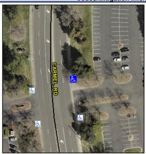
**CARMEL RD** Street 1 Name Stop Condition-Street 2 None Street 2 Name **ENTRANCE** Stop Condition-Street 1 None Possible Solutions: Remove & Replace Curb Ramp With **Two New Directional Ramps or** Equivalent. Surveyor Notes: N/A PROW/ADA: Not Found, R304.5.1, R304.2.2
