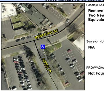
Street 1 Name Stop Condition-Street 2 Street 2 Name Stop Condition-Street 1 MONTFORD DR None **ABBEY PL** StopSign Possible Solutions: Remove & Replace Curb Ramp With Two New Directional Ramps or Equivalent. Surveyor Notes: N/A
