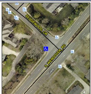
Street 1 Name Stop Condition-Street 2 Street 2 Name Stop Condition-Street 1 S WENDOVER RD None SEDGEWOOD CR StopSign Possible Solutions: Remove & Replace Curb Ramp With **Two New Directional Ramps or** Equivalent. Surveyor Notes: N/A PROW/ADA: Not Found, R304.5.1, R304.2.2, R304.5.3
