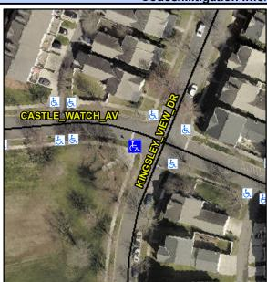
KINGSLEY VIEW DR Street 1 Name Stop Condition-Street 2 StopSign **CASTLE WATCH AV** Street 2 Name Stop Condition-Street 1 StopSign Possible Solutions: Remove & Replace Curb Ramp With Two New Directional Ramps or Equivalent. Surveyor Notes: N/A PROW/ADA: R304.5.1
