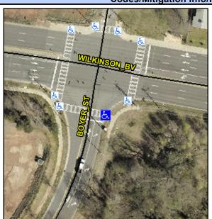
**BOYER ST** Street 1 Name Stop Condition-Street 2 Signal N/A Street 2 Name Stop Condition-Street 1 N/A Possible Solutions: Remove & Replace Detectable Warning System. Surveyor Notes: N/A PROW/ADA: R305.2
