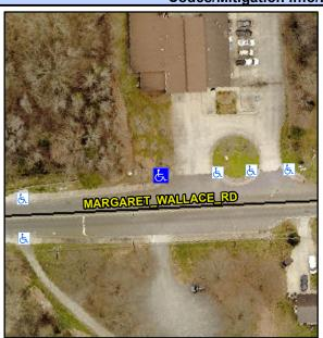
MARGARET WALLACE RD Street 1 Name Stop Condition-Street 2 None **ENTRANCE** Street 2 Name Stop Condition-Street 1 None Possible Solutions: Remove & Replace Curb Ramp With Two New Directional Ramps or Equivalent. Surveyor Notes: N/A PROW/ADA: Not Found, R304.5.1, R304.2.2
