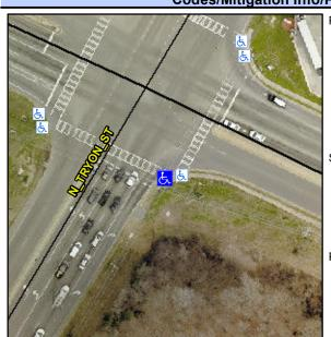
**NORTH TRYON ST** Street 1 Name Stop Condition-Street 2 Signal Street 2 Name N/A Stop Condition-Street 1 N/A Possible Solutions: Remove & Replace Entire Ramp. Surveyor Notes: N/A PROW/ADA: R304.5.1, R304.5.3
