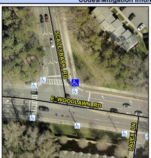
Street 1 Name Signal Stop Condition-Street 1 SCALEYBARK RD Street 2 Name Signal Stop Condition-Street 2 E WOODLAWN RD Possible Solutions: Remove & Replace Curb Ramp With Two New Directional Ramps or Equivalent. Surveyor Notes: N/A PROW/ADA: Not Found, R304.3.2
