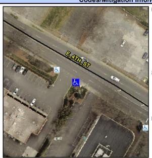
E 4TH ST Street 1 Name Stop Condition-Street 2 None Street 2 Name **ENTRANCE** Stop Condition-Street 1 StopSign Possible Solutions: **Remove & Replace Curb Ramp With Two New Directional Ramps or** Equivalent. Surveyor Notes: N/A PROW/ADA: Not Found, R304.5.1, R304.2.2
